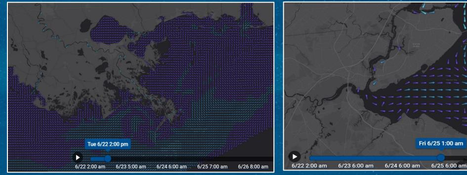
S-111 surface current data enables route optimization; Fuel reductions = emissions reductions and cost savings
